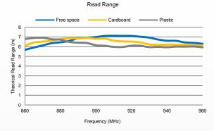
All the graphs are indicative: performance in real life applications may vary. The data has been determined based on calculations for transmitters with a 2W ERP output power level and an Impinj Monza R6 tag silicon.
